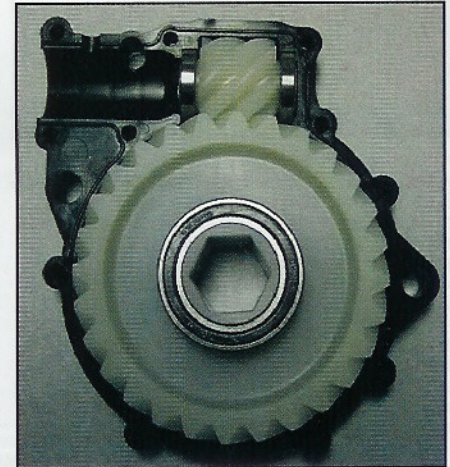
FIG. 12: THESE CROSSED HELICAL GEARS ARE USED IN AGRICULTURAL EQUIPMENT. IT WAS POSSIBLE TO REPLACE AN OLD-STYLE METAL CHAIN DRIVE WITH A LESS EXPENSIVE, SAFE, AND MAINTENANCE-FREE PLASTIC GEAR DRIVE AND FLEXIBLE SHAFT.
