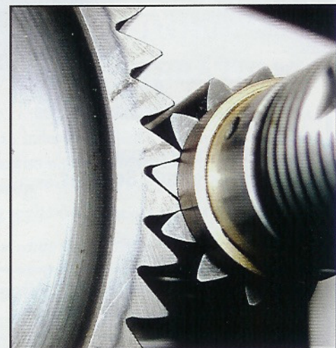
FIG. 14: IN THESE GENERATOR GEARS, APPLICATION OF THE ASYMMETRIC FOR THE EXPERIMENTAL GENERATOR GEAR DRIVE ALLOWED FOR A SIGNIFICANTLY REDUCED VIBRATION LEVEL.
