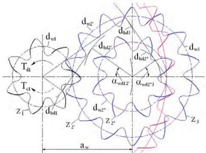
Figure 4: Epicyclic mesh with compound planet gears
