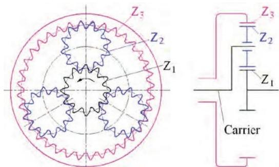
Figure 1: Epicyclic stage with singular planet gears; numbers of teeth:  $z_1$  — sun gear,  $z_2$  — planet gear, and  $z_3$  — ring gear
