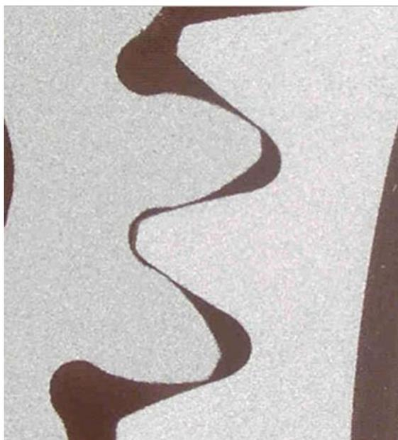
experimentally determine their single-tooth bending fatigue strength and scuffing resistance. The gear test specimens are presented in Fig. 14.
