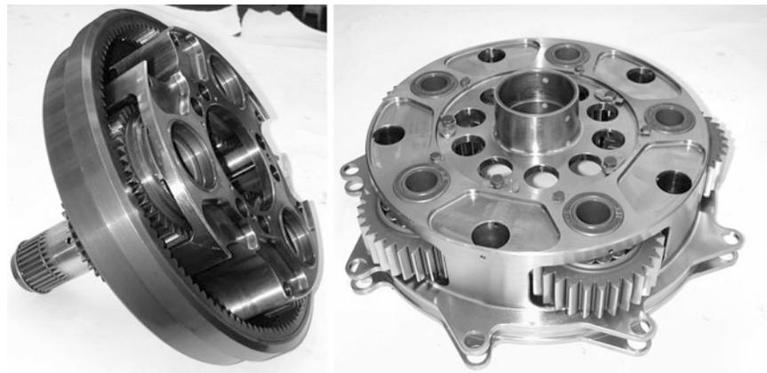
**Fig. 18** First and second stage assemblies
