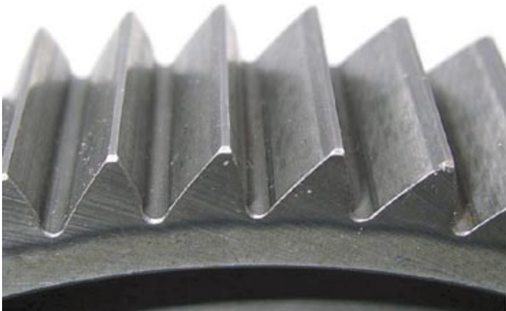
c) Experimental gear for aerospace application
